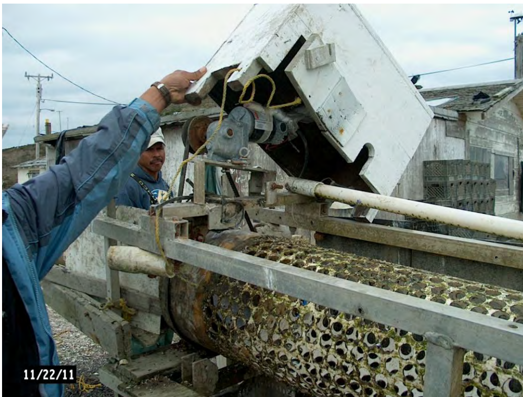
Photo 4. Oyster Tumbler Motor (and primary noise source)
